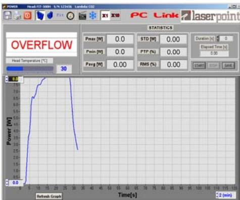
Every time the laser power or energy exceeds the head full scale an OVERFLOW alarm is displayed as shown in the picture .
